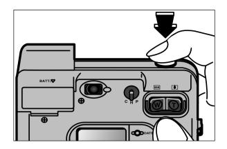
When the shutter trips, the flash fires and the film advances to the next frame.
